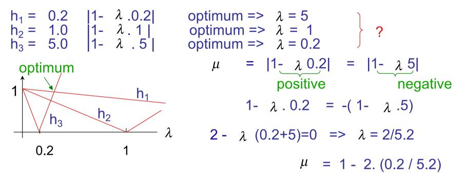
Only ~ 8% decrease of the error, per iteration ! Hundreds of iterations will be needed to reach a reduction of the error by 1000 or more.
