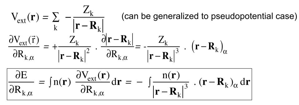
Forces can be computed directly from the density ! Also, similarly, stresses. => Optimization of geometry (lattice parameters and atomic positions)
